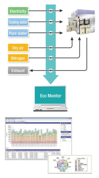
Monitors electricity, exhaust, water (cooling water and pure water), dry air and nitrogen as comprehensive energy during the actual operation of the equipment in accordance with SEMI S23\*.
