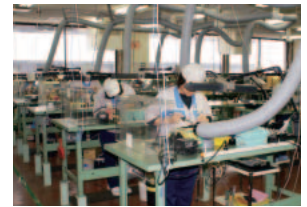
▲ Lead-free soldering production line
