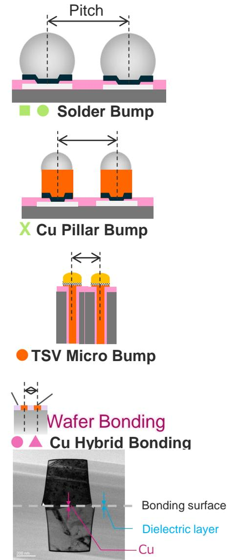
Introduction of wafer bonding technology accelerates further reduction of pitch
