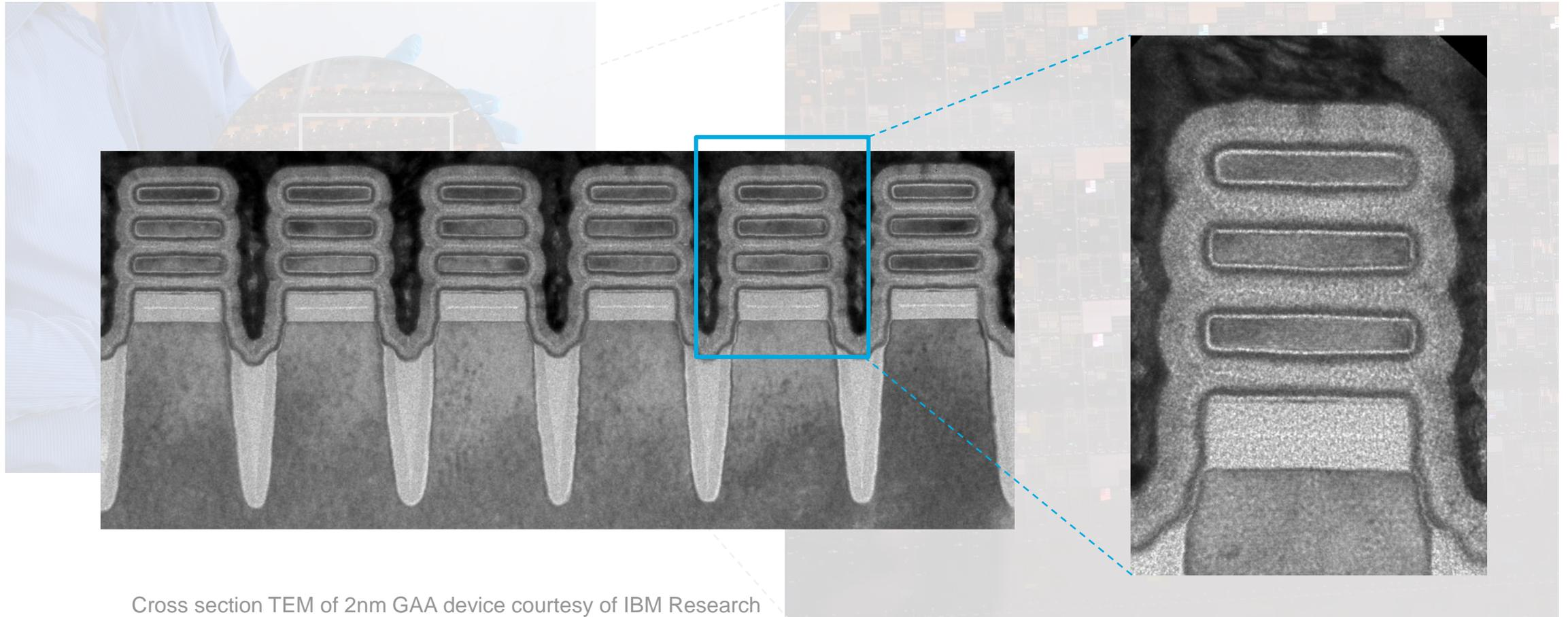
Cross section TEM of 2nm GAA device courtesy of IBM Research
