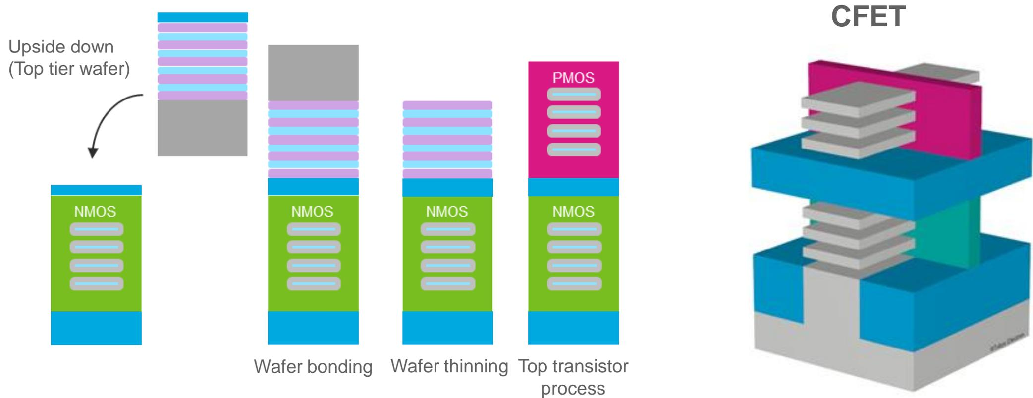
Low distortion wafer-to-wafer bonding technology and substrate film thinning technology are necessary for scaling booster technology
