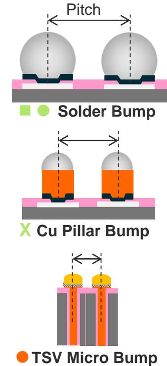
Introduction of wafer bonding technology accelerates further reduction of pitch
