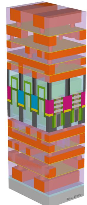
Low distortion wafer-to-wafer bonding technology and substrate film thinning technology are necessary for scaling booster technology
