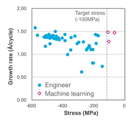
Process: PE-ALD SiO<sub>2</sub> deposition Target: film stress → between -100MPa 0MPa
