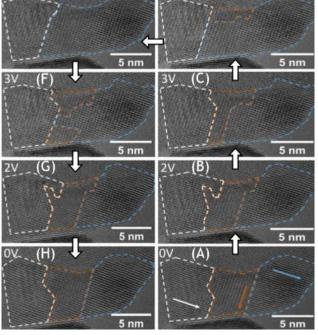
Multi-source supply enables controllable film composition, making possible the formation of various functional films In-situ TEM measurement with simultaneous voltage cycling of antiferroelectric ZrO. Crystal grains grow and shrink by field driven domain wall migration as the voltage cycles from  $0V \rightarrow 4V \rightarrow 0V$ .
