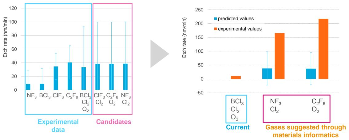
Gases with higher etch rates than before were suggested using machine learning
