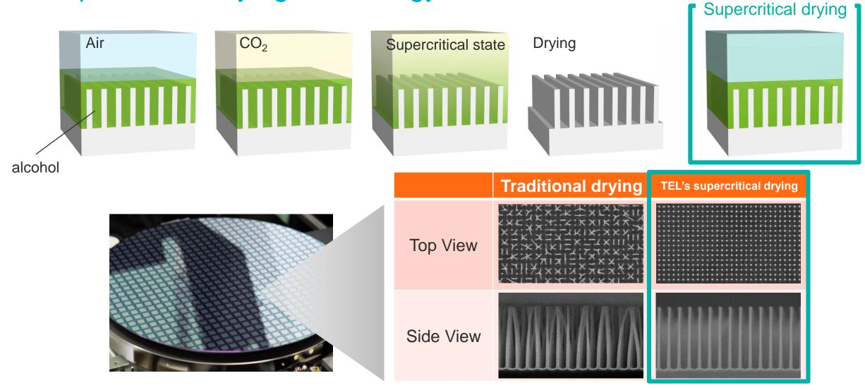
Supercritical drying technology prevents pattern collapse
