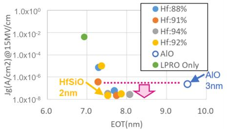
Leak current of HfSiO 2nm-thick is smaller than that of AIO 3nm-thick on TEL MOS capacitor
