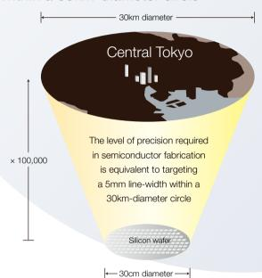
LSI circuits of approximately 1cm² are formed from disc-shaped silicon wafers 30cm in diameter. The most advanced manufacturing technologies enable fabrication of transistors in an LSI circuit on a scale as small as less than 50 nanometers (nm),\*1 allowing several hundred million transistors to be incorporated into one LSI.
