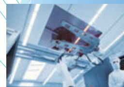
Oerlikon Solar's KAI PECVD system
